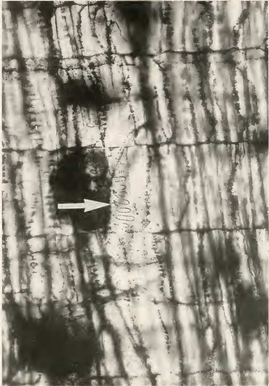
Fig. 10. Radial section (BSP 1964 I 486). Vessel-ray pitting gash-like (arrow) or oval-shaped. Note: All vertical walls of the upright ray cells have disjunctive cell walls; x 360, photo D. GROSSER
